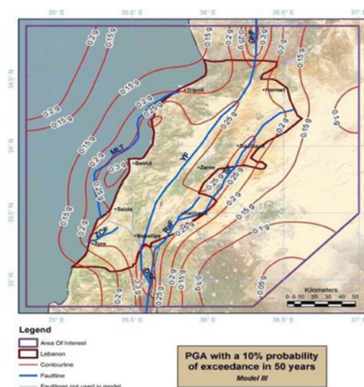
Figure 25 Seismic hazard map of Lebanon, distribution of PGA for 50-year period (return period of 475-years).
